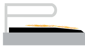
elevated cubicle with KRAIBURG mat
