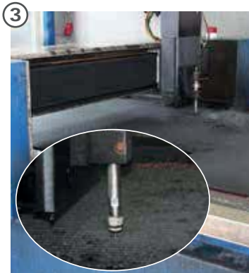
3 based on the CAD created drawing, the slits are cut exactly into the mats with innovative water jet technology
